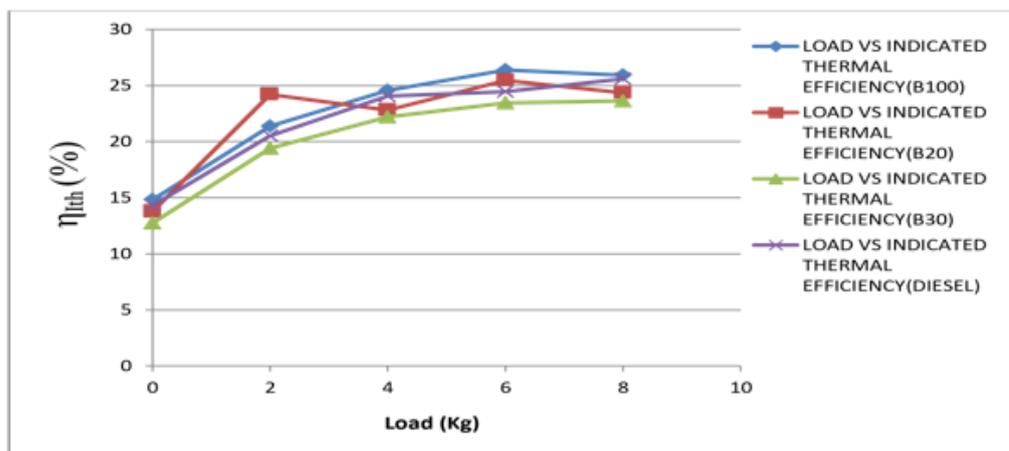
Fig.6 Load vs thermal efficiency
