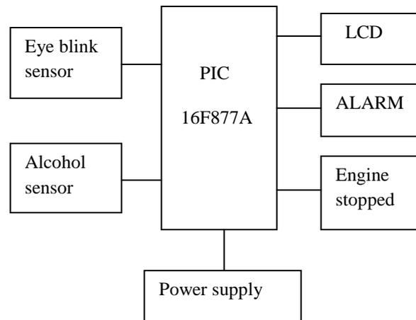
Figure 01: Block Diagram of the System
