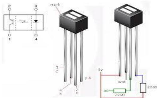
Figure 02: Pin Diagram of Eye blink sensor
